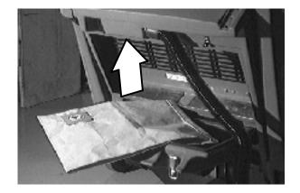
Latch the filter compartment door. Fully insert the vacuum wand into the machine.
