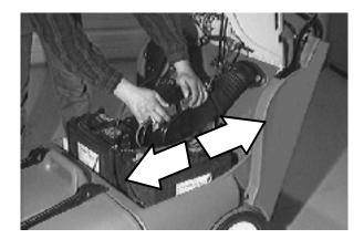
8. Plug the charger connector into the battery connector.
