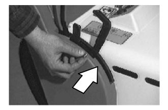
4. Ensure the battery bags are in place. Do not remove battery bags from machine.
