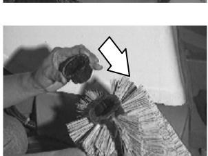
5. Pull the main brush out of the machine through the hopper opening.
