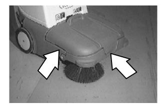
With one person on each side, lift the debris hopper out of the machine.
