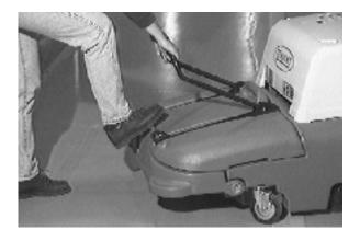
Lift the hopper out of the machine and onto the wheels. Transport the hopper to the location where debris is collected.
