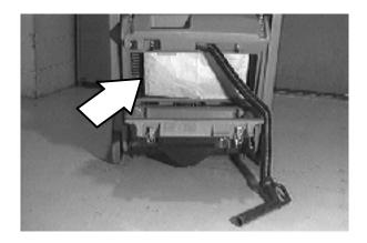
To access the bag filter, remove the vacuum wand and unlatch the filter compartment hooks.
