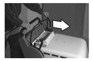
3. Gently squeeze the clutch handle to move the machine forward.
