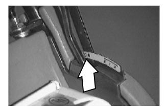
*REVERSE:* Move the directional control lever to the left, then one position forward from the PARK position. The machine will move backward when the clutch handle is squeezed.
