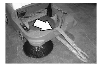
5. Block the machine tires and place the directional control lever in Park. Tie down the machine to the truck or trailer before transporting.
