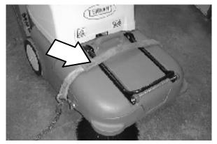
6. If the loading surface is not horizontal or is higher than 380 mm (15 in) from the ground, use a winch to unload machine.
