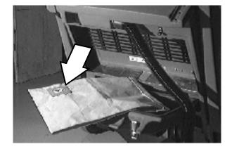
The vacuum inlet tube is located at the top of filter compartment, on the inside of the machine.
