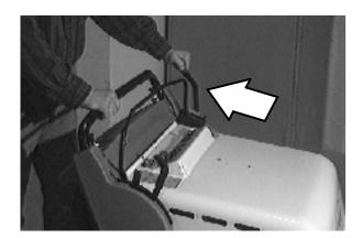
5. Shake the panel filter by pressing the filter shaker switch. The shaker motor will operate for 15 seconds before stopping.
