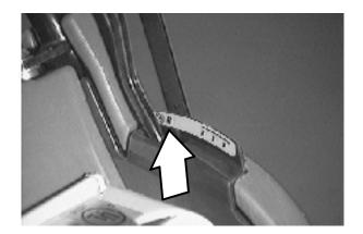
*NEUTRAL:* Push the directional control lever halfway between the REVERSE position and the SECOND SPEED position. The machine will not move forward when the clutch handle is squeezed while in NEUTRAL. Do not leave the machine powered on in NEUTRAL while the machine is unattended.
