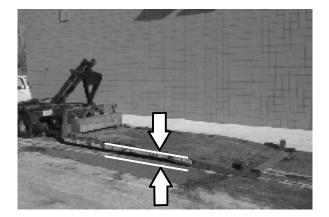
To winch the machine onto the truck or trailer, remove the hopper and place a strap through the front frame of the machine. Make sure the machine is in neutral and is centered.
