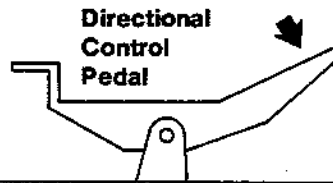
DIRECTIONAL CONTROL PEDAL IN "FORWARD" POSITION
