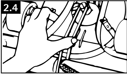
2.4 Place belt on pulley. Side of belt nearer cleaner should be in line with projections on bottom of cleaner. Replace bottom plate, by putting knobs on front of plate into wire holders on cleaner. Check to see that latches are pushed back and will not be covered by plate. Position bottom plate over agitator and latch securely.
