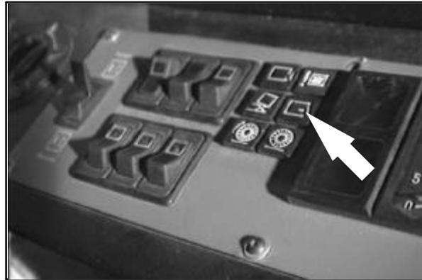
2. Make sure the hopper tilt light is off. If the hopper tilt light is on, lower the hopper till the light goes off.
