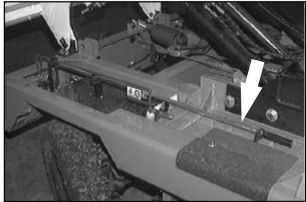
3. Close the vacuum door with the vacuum wand door tool. Place the tool back in its storage location under the hopper.
