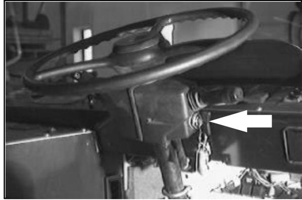
2. Raise the hopper slightly to relieve pressure on the hopper support pins.
