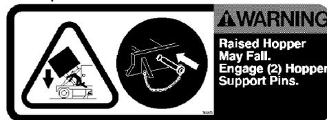
**HOPPER SUPPORT PINS LABEL (High Dump Model) -**
