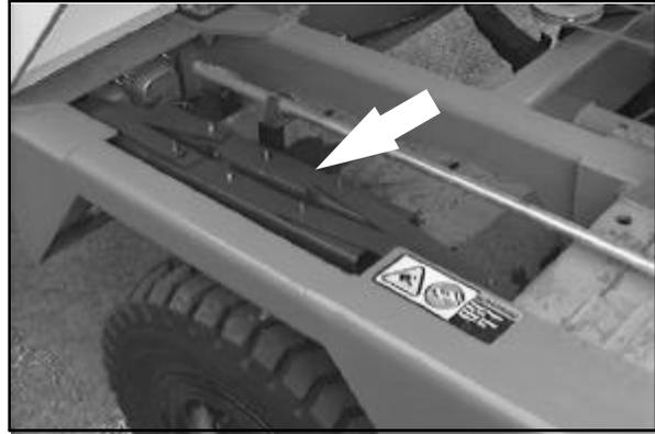
For machine serial number 001710 and above, remove the hopper support pin and fasten it in the storage location on the right rear fender.
