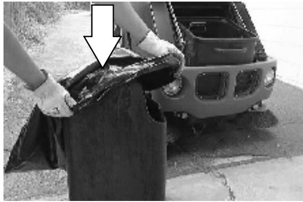
15. Insert new bag and liner, or debris hopper if not using bags, back in the machine.
