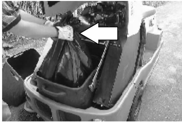
12. Remove and empty the debris hopper if bag liners are not being used. Wet debris can be heavy. If the hopper is heavy, get help to lift it and dispose of the debris.
