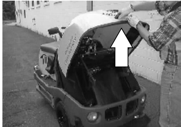
6. Pull on the cover prop rod to lock cover in open position.
