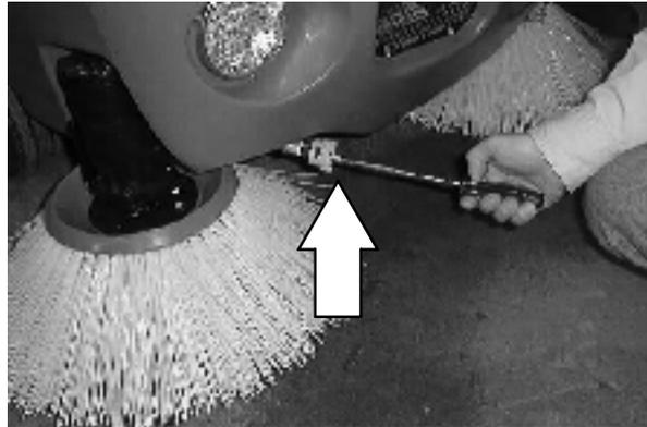
9. The adjusted side brush spray pattern should form a wide "V" pattern in front of the machine, intersecting in between the brushes.
