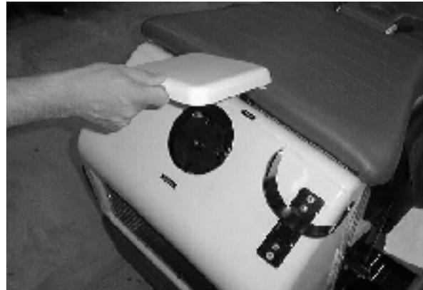
4. Lift the steering assembly off the front notched steering plate. Unfold the steering assembly back over the machine seat.
